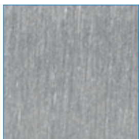
fronts in stainless steel (1.4301), brushed surface
